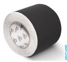
GTB65™ is a professional grade reinforced 30 micron aluminium foil tape in a matt black finish. This foil / scrim laminate with a bi-directional 5mm x 5mm reinforcement is coated with a high performance acrylic pressure sensitive adhesive and protected by an easy release silicone paper.
